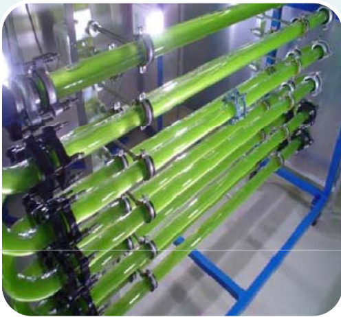
Tubular photobioreactor High efficiency but high cost
