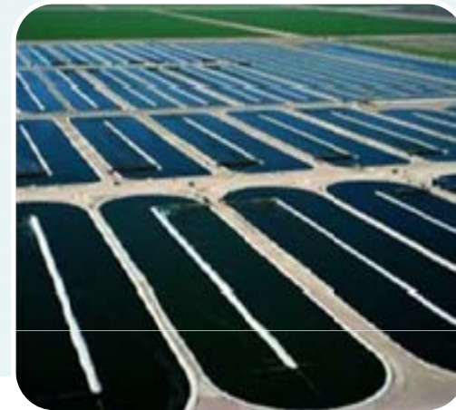
Raceway pond Low operation cost but low growth yield
